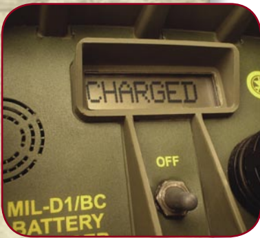
MIL-D1/BC DISPLAY SHOWING PART OF THE "BATTERY CHARGED" MESSAGE
