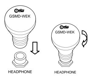
Switch on the detector: within a few seconds the Earphone will automatically pair to the detector. The LINK indicator turns on and the Earphone starts replicating the detector acoustic signals.
