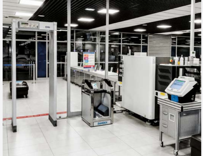
Passenger Screening by Walk-Through Metal Detector (WTMD), Shoe Scanner (SAMDEX) and passenger body control through Explosive Trace Detector (ETD)
