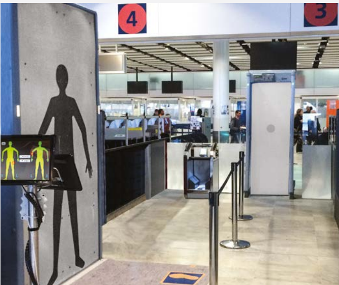
Passenger Screening by Walk-Through Metal Detector (WTMD), Shoe Scanner (SAMDEX) and passenger body control through SECURITY SCANNER
