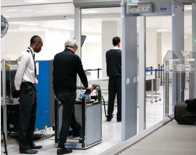
Passenger Screening by Walk-Through Metal Detector (WTMD), Shoe Scanner (SAMDEX) and passenger body control through PAT-DOWN
