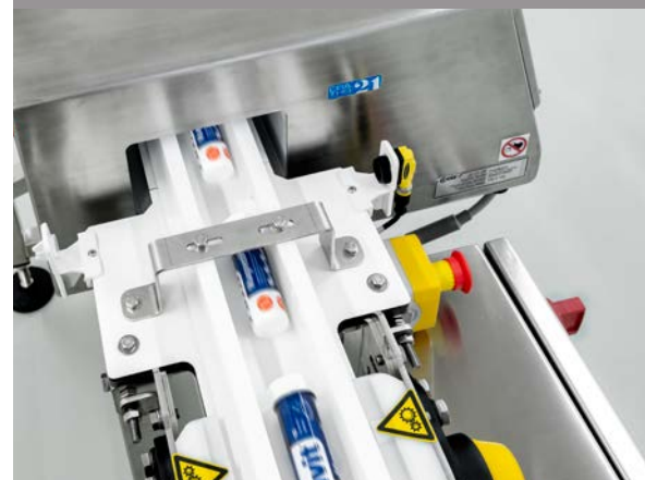
THS/FBB for plastic tubes and sanitary packages inspection.
