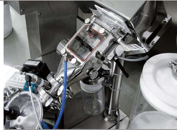
THS/PH21N-WIP: Wash-in-Place Metal Detection System.
