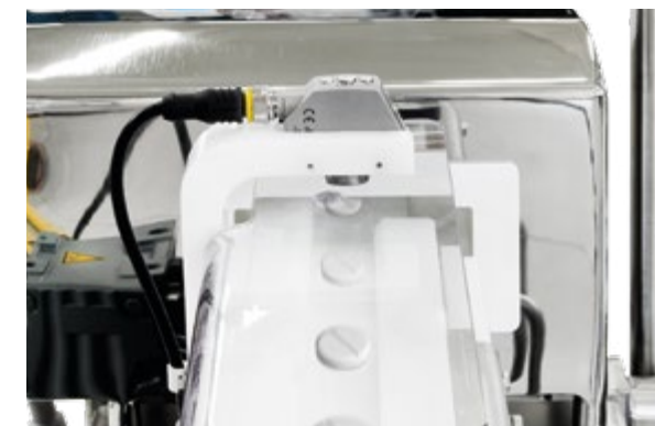
THS/FBB for plastic tubes and sanitary packages inspection.
