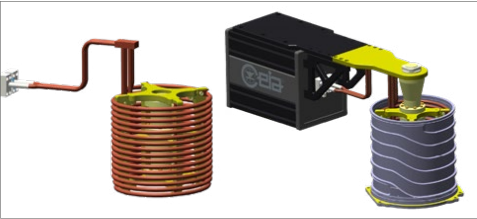
Detailed electromagnetic modeling and analysis to achieve the customer's heating requirement
