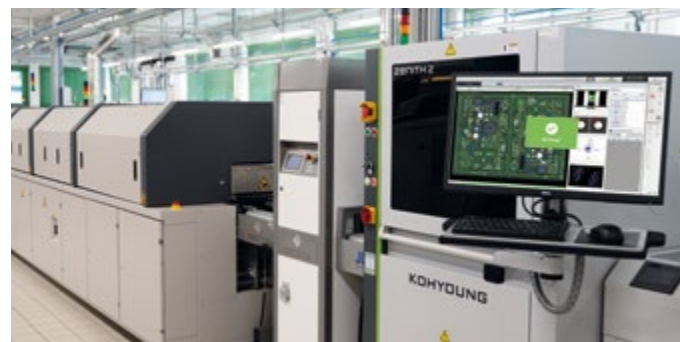
In-line automatic optical inspection (AOI) of electronic boards
