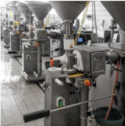
THS/PLV-MEAT 21 Series Pass-through piping Integrated System with ejection valve for applications on meat vacuum filler filling machines.
