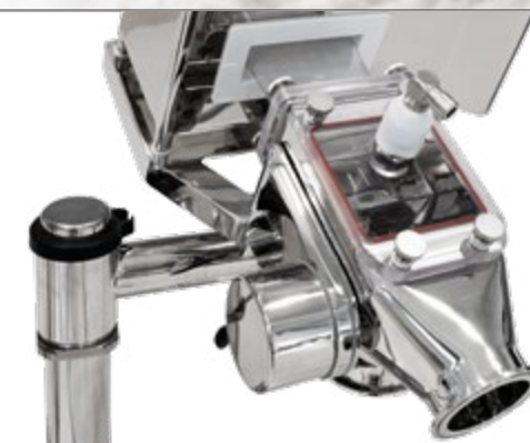
THS/PH21N-WIP Wash-in-Place Metal Detection System.
