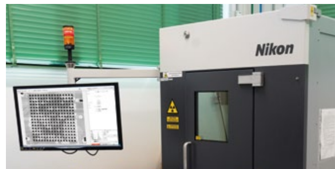
X-ray inspection of electronic boards and components
